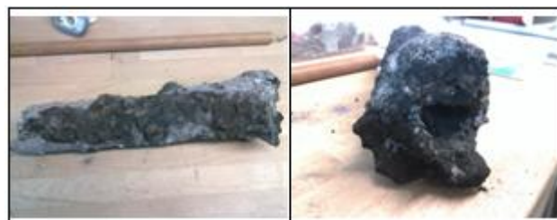
Figure 5: Remnants of a damaged 10KV cable. The above cable was operational and carrying nominal voltage/current in the depicted state until the fault was discovered by unrelated excavation work. The "lump" on the cable remnants is a piece of granite stone melted around the cable.
