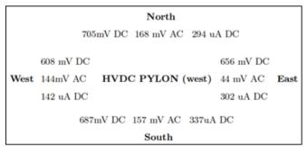
**Figure 11**: The HVDC pylon is a point source of both AC and DC leak current, although supplemental measurements with differential magnetometer indicates that a large (but unquantifiable with present technology) part of the leaked stray current originates from the wind turbine.
