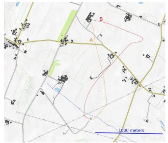
**Figure 1**: Red and orange dashed lines denotes two different magnetotelluric anomalies. There are no obvious reasons as to their path through the landscape, with the single exception that the path of both magnetotelluric anomalies are strongly perturbed by steel lattice pylons for the 285kV "Kontiscan"
