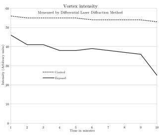
**Figure 4:** Both laser beams are projected onto similar PVarrays and subjected to the same data acquisition and analog/digital conversion. Only difference is that the exposed beam traverses the magnetotelluric anomaly, whereas the "control" does not. The two graphs will naturally start at different values, as the PV array and laser
