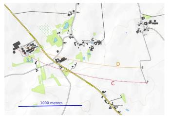
Figure 2: Red and orange dashed lines denotes two different magnetotelluric anomalies. We note that there is evidence of significant perturbation of their paths by storage tanks at a biogas plant located east of the farm buildings. Map data: © OpenStreetMap-Mitwirkende, SRTM | Kartendarstellung: © OpenTopoMap (CC-BY-SA)
