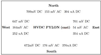
**Figure 12:** The second HVDC pylon is also a point source of both AC and DC leak current. As for the other pylon, we conducted supplemental differential magnetometer measurements, indicating a large current travel from the wind turbine to the HVDC pylon, indicating that the leak current measured from the HVDC pylon had its original source in the wind turbine.
