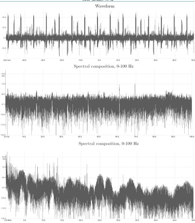
Figure 3: The waveform composition is, per present empirical observations, unique for each source of magnetotelluric anomalies. We note that the waveform often contains artifacts with a plausible origin stemming from leak current patterns from electrical infrastructure or appliances with a pulse-modulated current intake.
