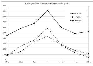
**Figure 12:** Cross gradient analysis for magnetotelluric anomaly "B" indicate a rather substantial current/voltage gradient from the magnetotelluric anomaly towards the ground clamp at the electrical transformer.
